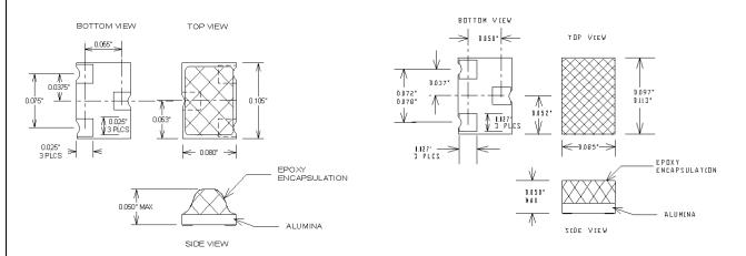
Packages are designed with wrap-around metalized castellations for superior assembly results.
